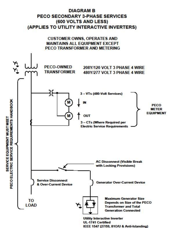
NOTE: ALL GENERATION SOURCES TO BE CONFIGURED AS A SOLIDLY GROUNDED-WYE CAPABLE SUPPLYING CUSTOMER SINGLE-PHASE LOADS CONNECTED PHASE TO NEUTRAL. SEE AC SCHEMATIC FIGURES X, Y & Z.
