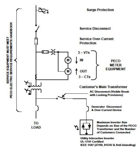
NOTE: ALL GENERATION SOURCES TO BE CONFIGURED AS A SOLIDLY GROUNDED-WYE CAPABLE SUPPLYING CUSTOMER SINGLE-PHASE LOADS CONNECTED PHASE TO NEUTRAL. SEE AC SCHEMATIC FIGURES X, Y & Z.
